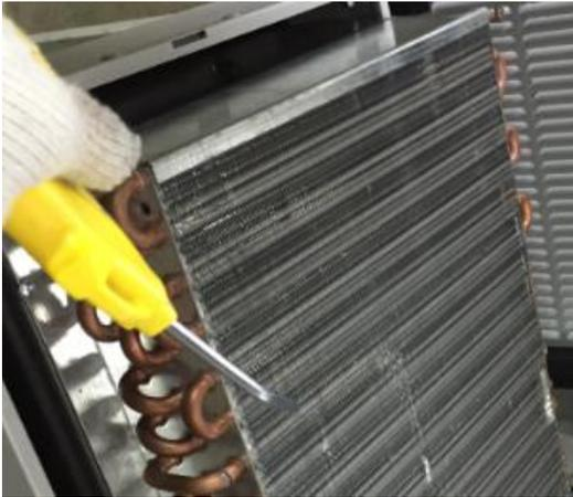
Figure 25: Clean the heat exchanger using compressed air
